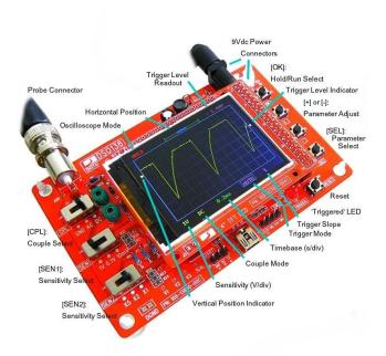
Timebase (s/div): Timebase is the horizontal axis of the display. As we discussed regarding the voltage (Vertical) axis, each division is the dotted square, but horizontally, and each dot represents 0.2 of the next division. When selected, Timebase appears green in a blue box. When the Parameter Adjust buttons are pressed, its value changes from the lowest of 10us to the highest of 500s, in the following values:
