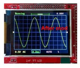
This is caused by excessive loading of U2B by the potential divider R6/7/8. The solution is easy: Replace R6, R7 and R8 with resistors ten times greater in value, i.e. R6 = 3k, R7 = 1.8k, R8 = 1.2k. The right photo shows the waveform after the modification.
