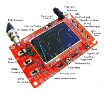
DC Power: Connect a 9-12Vdc power source to the DC jack or attach a 9Vdc battery's leads to the white connector beside the power jack. Do NOT exceed +12Vdc, or U5 will get hot!
