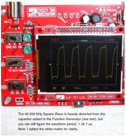
As you can see, I'm using our DL4YHF2 Frequency Counter, our XR2206 Function Generator (set for a  $40.5~\mathrm{KHz}$  square wave), and our new DS0138 Oscilloscope to show the
